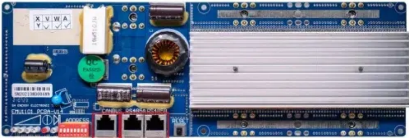
RS485 Communication between battery and inverters Baud rate:9600bps
